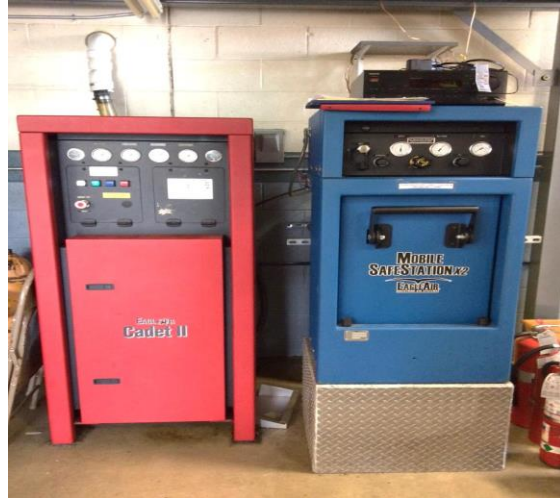
RED - EAGLE AIR COMPRESSOR MFG. DATE 03-11-2002 401.7 HR. 01-11-2023 BLUE – EAGLE AIR CYLINDER FILL STATION MFG. DATE 06-28-2013
